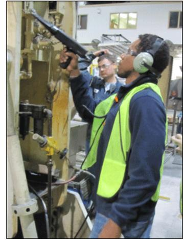
*KPPC Associate Engineer Brandon Burfict uses ultrasound equipment to detect compressed air leaks during an environmental sustainability assessment.*
