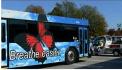
*This hybrid electric bus, operated by the Transit Authority of River City – TARC – in Louisville, was one of the vehicles on display at the main workshop site in Lexington on Nov. 10. In addition to improved emissions, the bus gets better fuel economy than standard buses and has lower maintenance costs.*
